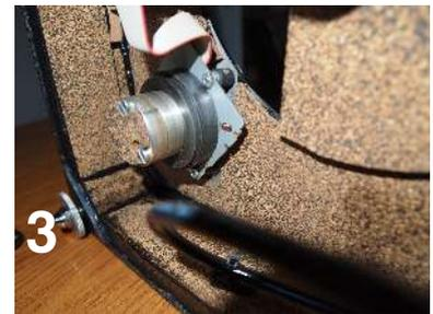
4. Floppy drive electrics mounted on steel bracket and side of case plus damping.
